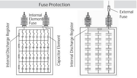
A - Capacitor with Internal element fuse
